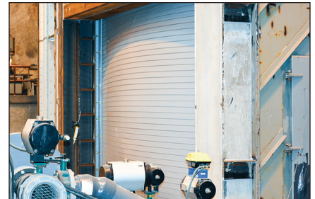
Subjected to both a positive and a negative 255 mph windload.
