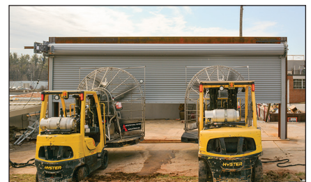
Fully functional with no damage or deformation after subsection to a 110 mph wind load.
