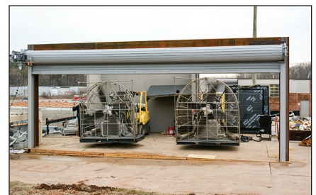
Fully operational while subjected to a sustained 110 mph wind load.
