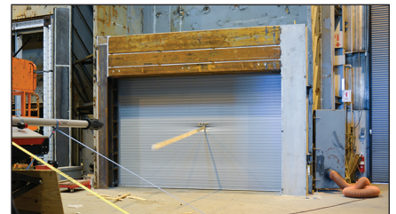
Missile impact test proves ability to withstand windborne debris from a hurricane or tornado.
